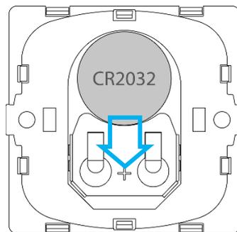
Figure 1: Inserting battery
