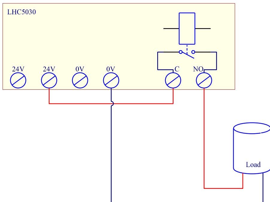
Above schematic outlines an example of how the 24V supply output, together with a relay output, can be used to control a load.
