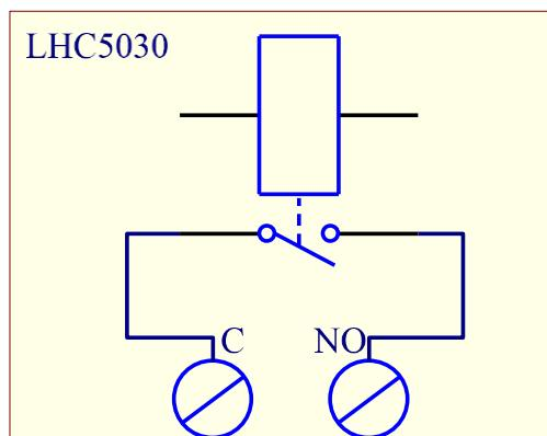
Above schematic outlines how the relay outputs are implemented internally.
